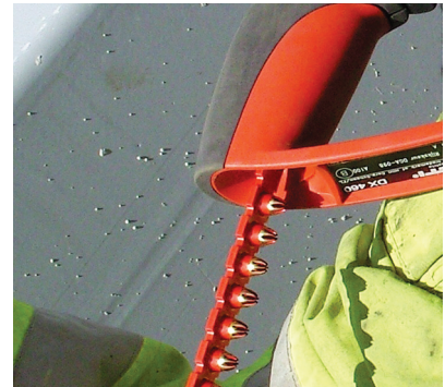
Use Red cartridges for steel. Black cartridges for harder or high strength steel
