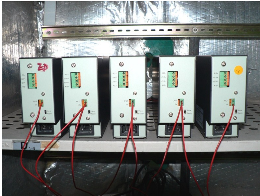
Figure 3 Setting of Master and Slave connections at the rear panels of 5 units of SSP-7080 modular power supplies
