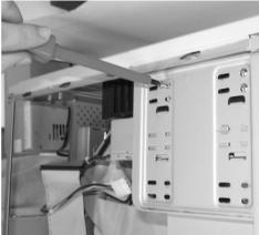
Once you have placed the PC bay into the 5.25" bay, you will need to secure it in place. Align the front of the PC bay so it is even with your other 5.25" devices. Once the PC docking bay is in line with other devices, you can make minor adjustments and use the eight included screws to secure the bay into place as shown above.
