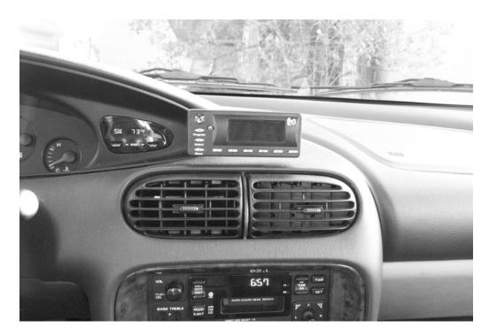
It is suggested that the remote LCD be installed as low as possible, especially in cars that allow a lot of sun. Installing the remote LCD low on your dash will allow you to easier reach the buttons, and will also reduce glare caused by the sun, increasing visibility.
