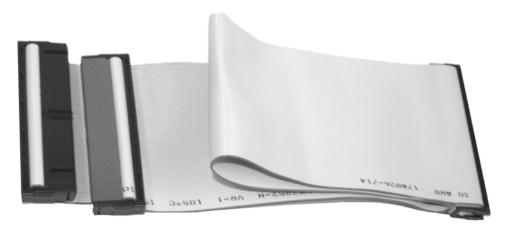
Once you have located the IDE cable that goes to your computers hard disk drive, you will need to follow it back to the computers main board. On this board you will either see another IDE cable of the same size next to the main one, or you will see a slot in the main board in which an IDE cable can be plugged in. If there is an empty slot in the main board please follow the directions in section 3.1, if there is a cable, see section
